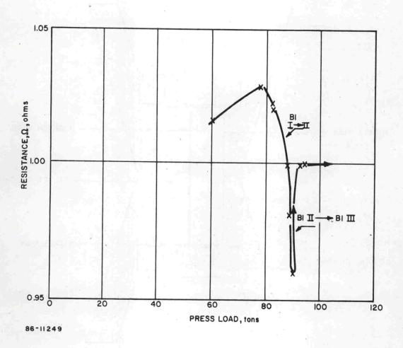
Figure 4 CALIBRATION (PRESSURE)
